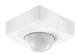
A head for heights. Powerful reach. Reliable. IS 3360 MX Highbay motion detector – ideal for high ceilings in industrial buildings or commercial properties. For mounting heights of up to 14 m. High-precision 360° infrared sensor. Maximum reach: 18 m. For watching over up to 1000 sq.m. Available as square surface-mounted and concealed version. DALI-2 Input Device enables sensors to communicate collected sensor data to higher-level lighting management systems.
